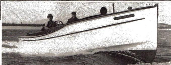
Jr., of New Bedford, Mass. She is 29 feet in length, with a beam of 7 feet 2 inches and an extreme draft of 26 inches. The motor installed is a 6-cylinder, 60 h.p. Loew-Victor with full automobile control, including electric self-starter, electric
