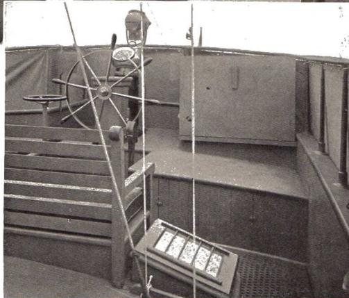
By eliminating brass fixtures and by laying canvas over the decks, the labor of keeping the boat clean has been reduced to a minimum.
