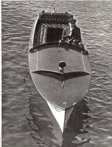
serves to prevent any water from finding its way into the engine compartment, and an air scoop provides ventilation for this section. The boat measures exactly 21 feet in length by 5 feet beam.
